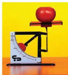
Figure 2.18 Lever balance with circular scale
