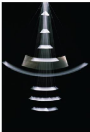
Figure 13.20 Time-exposure photographs of Barton's pendulums with light damping, taken end-on. The longest arc, in the middle, is the driver.
