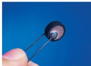
Figure 11.7 Thermistors are useful temperature measuring devices
