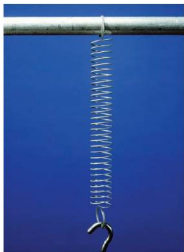
Figure 6.9 The spring stores energy as it is stretched, releasing the energy as it returns to its original shape.
