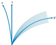
Figure 26.3 Deflection of \alpha - and \beta -particles and \gamma -radiation by a magnetic field into the page
