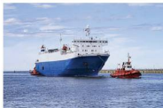
Figure 6.3 The useful work done by the small tug-boat is found using the component of the tension in the rope along the direction of motion of the ship.
